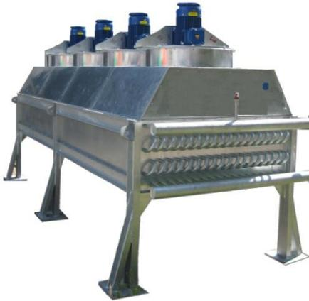
The cooler as shown in the picture is a so called dry cooler for cooling of compressor oil. The cooler is equipped with explosion proof fans and motors and is designed for an ambient temperature of 45 °C. The design is according ASME and the witness test was carried out by LRS.
